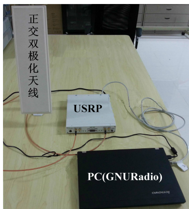
图 11 GNURadio+USRP 组成的软件无线电平台 Figure 11 The GNURadio+USRP based software radio platform
