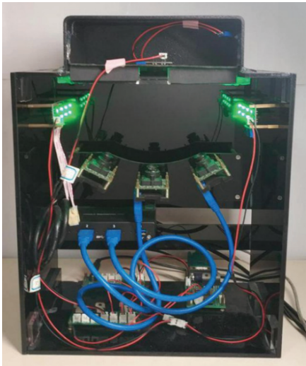
图 8 启动中的采集设备, 设备打开摄像机, 并开启可见光源, 先采集三个不同角度的指折痕图像 Figure 8 Acquisition device in startup. The device turns on the camera, turns on the visible light source, and collects finger crease images from three different angles
