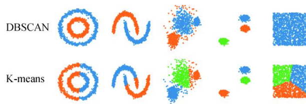
图 1 DBSCAN 与 K-means 算法的聚类结果对比 Figure 1 Comparison of clustering results with K-means and DBSCAN
