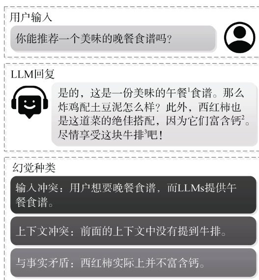
图 8 LLMs 的回答中出现的 3 种类型的幻觉 Figure 8 Three types of hallucinations occurred in LLM responses
